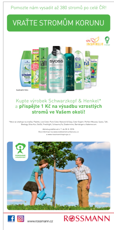
Top card on display, offset printing (stochastic grid), 150g glossy chalk on full board with counter-laminated backing.
