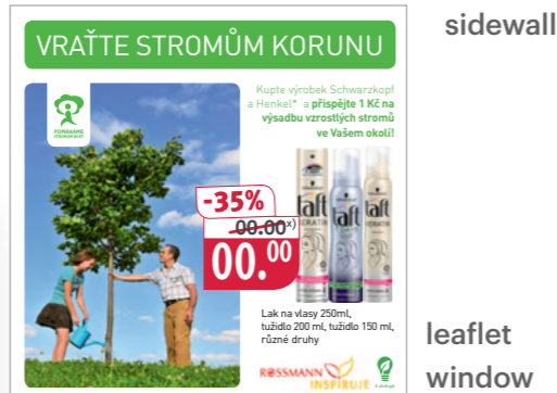
Top card on display, offset printing (stochastic grid), 150g glossy chalk on full board with counter-laminated backing.
